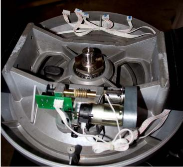
Next, remove the nut and washer using a 45mm wrench (if you have one) or channel lock pliers. Peel off any Loctite from the nut and set aside.
