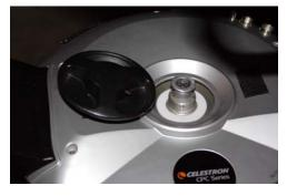
Remove the 5 screws from the plastic base cover and pop the cover off. Then disconnect the 5 cable straps. You may want to label them to make sure you reconnect them properly later on.
