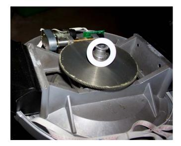
Next, remove the clutch plate. There are 2 set screws (2.5mm), on either side and a bolt (5mm) with a lock washer. Remove then and Peel off any traces of Loctite and set them aside.
