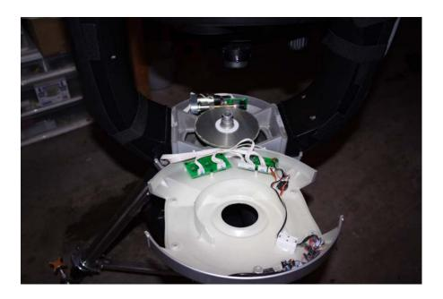
Next, remove the plastic clutch washer and lift up on the main gear to remove it. You may need to release the tension from the worm gear assembly. Just push against it to compress the spring and then lift the main gear.
