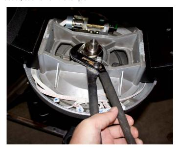
The rest is pretty simple. Just put the rest of the parts back in place. Put a bit of Loctite on the 2 set screws and bolt.
