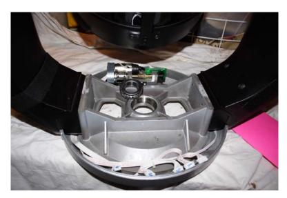
Insert the bearing back into the fork assembly. Now it's time to grunt.
