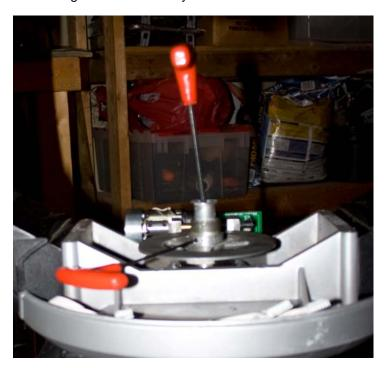
Put a bit of synthetic grease on the main gear teeth. Not too much! Then place the gear over the shaft. You will need to push the worm gear & motor assembly back to allow the main gear to seat itself against the friction plate.
