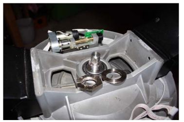
Now it's time to lift the fork assembly and reveal the nylon bearing balls.
