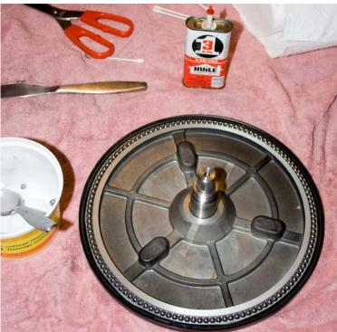
Now it's time to prepare the steel bearing balls. I dumped a bag of 100 into a container and then counted out 22 more from the other bag. I did not count to see if there were really 100 in the 1<sup>st</sup> bag but I am assuming that there were a few more than 100 because I had 4 left over after filling the channel.
