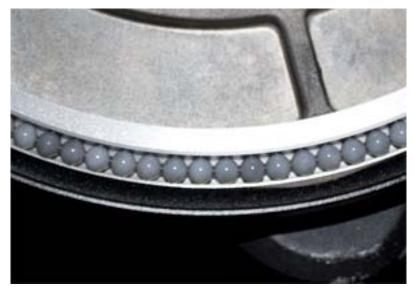
A few days earlier I attempted to fix my problem with some lubricant with the existing nylon bearings. It did reduce roll resistance but did not make the problem go away. This is the bottom of the fork assembly. It is basically an inverted cone. The arrow in the photo points to the point where the bearing balls touch the fork assembly. It is not a grove, just the marks made by the bearing balls.
