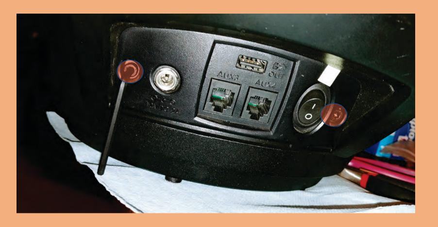
12) Remove the Allen screw left of the power in port and to the right of the power switch. Place screws in small zip lock bag and label. The white tape you see is glow in the dark tape to help locate the power switch in the dark.
