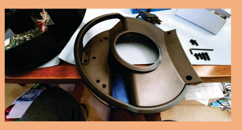
5) Once you remove all the bolts you will see that the base tray is in two pieces. Separate these two and put each in a large zip lock bag.
