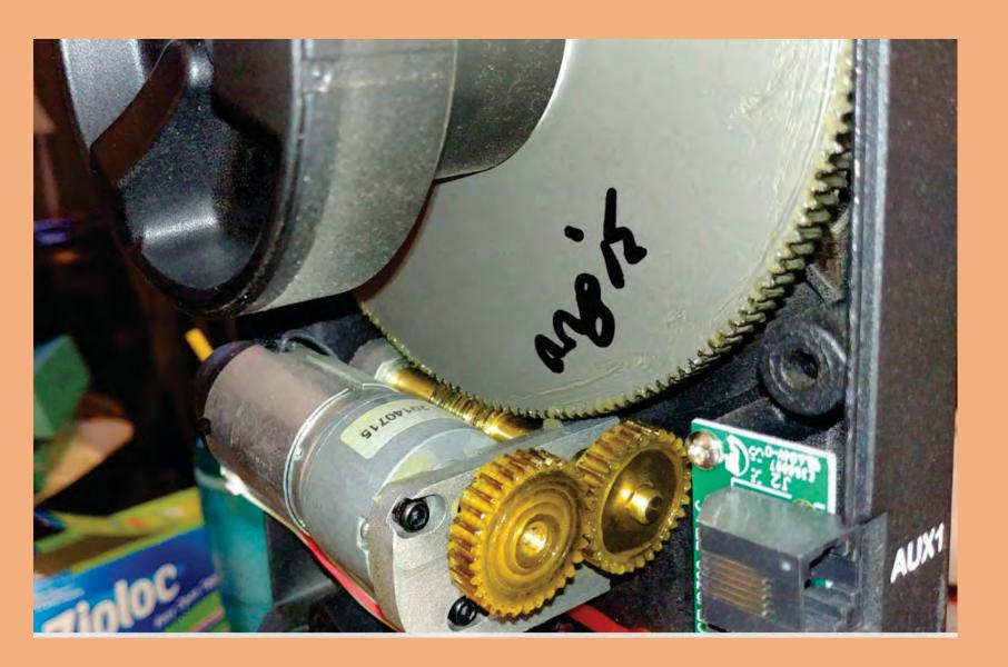
14) From here as you did during azimuth base disassembly, you can remove the clutch knob and lift off the big gear wheel.
