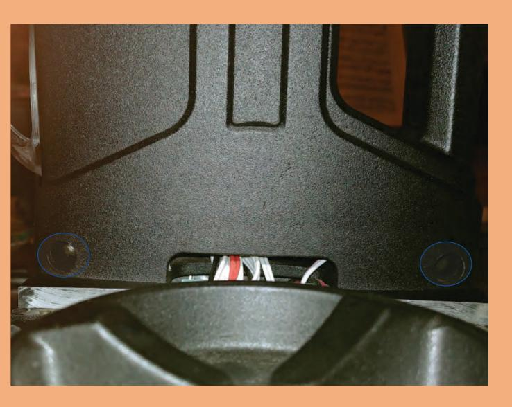
7) Start the screws at the inboard base. As you can see, you need to install these two screws before installing the azimuth base as the back of the base covers these two holes.
