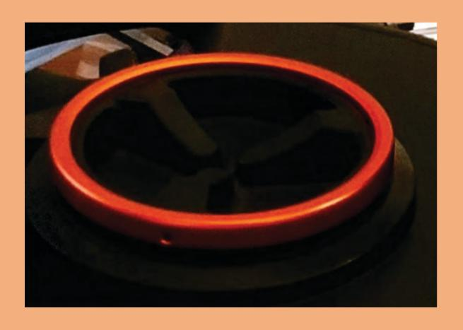
2) Using small Allen wrench loosen the **three** Allen screws from both the azimuth ring and the altitude ring. Please each ring in a zip lock bag.
