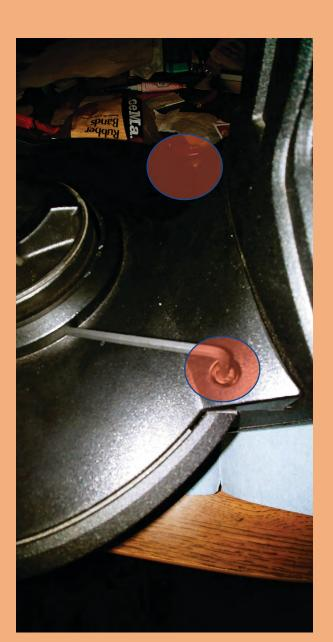
4) Use an Allen wrench to remove the **four hex Allen** screws at the base as well as **two hex Allen** screws close to the mount arm.
