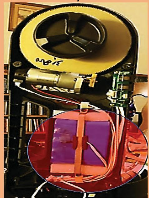
13a) Once you remove the outboard arm cover, you can see the battery and have clear access to it. There are a couple of threads that pertain to getting a replacement battery:
