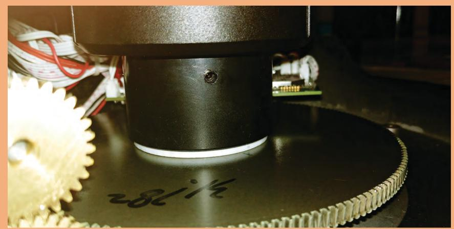
9) Here you see the main gear, the circuit card, the Azimuth clutch knob with the hex Allen screw shown and the white spacer. Be sure stall the a) main gear first, carefully seating on the base. B) Install the clutch knob and tighten the Allen Screw just enough to ensure that you can turn the clutch knob, tighten and loosen and the clutch knob stops. C) Then install the circuit cart with the four Phillips screws.
