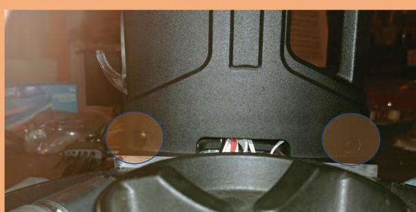
11a NOTE: There are two screws behind the azimuth tray. You need to remove the tray as discussed in slides 4-7.
