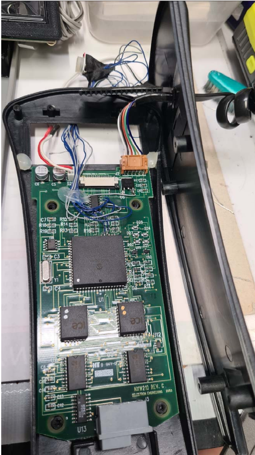
There's the trim pot at the top covered in black cloth tape. And the hot glue securing the wiring to the PCB. The black chip at top right is a 5V voltage regulator (a good place to get +5V from).
