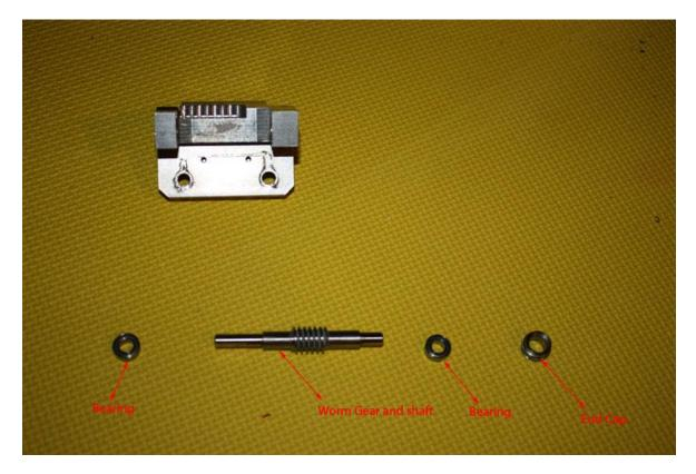
The bearings seemed to be fine, so I cleaned the worm/worm shaft, and put everything back to together, tightening it until the worm rotated roughly, and then backing it off until it was smooth again. I reassembled everything except the fork arm cover, and tried a few complete declination rotations with the hand controller. No roughness anywhere!
